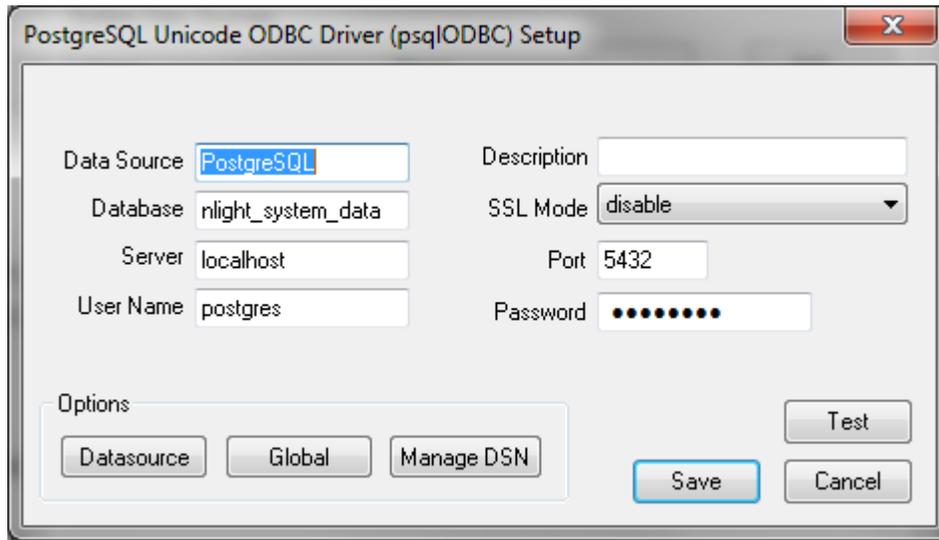
Select **Save**. Note, the Data Source name value as this is the field that must be entered into SensorView later. Note that pressing the **Test** button will fail with “database not found” until step 3.1 has been completed.
